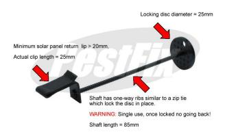
2.3.2 Roof covering: Kink the wire mesh as per installation instructions prior to offering up to solar panel frame. Then slide over sliding Solar Panel Bird Exclusion Clip and lock in position using non-return disc. No mechanical fixings will be necessary
