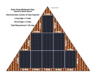
This non-penetrating system is fast and easy to install, and can be removed for service. Replacement Solar Exclusion Clips will be required for reinstatement after service.
